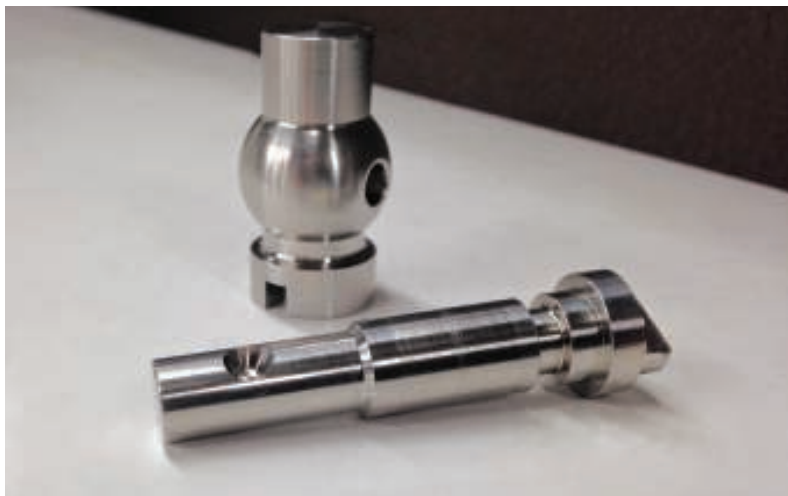
FIGURE 3. Stainless steel provides many beneficial properties for valve internals, but this material can pose challenges for machining processes
