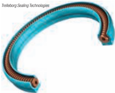
FIGURE 3. A PTFE-based sealing product, Turcon Variseal Ultra-Clean from Trelleborg, was developed to stand up to the harsh environments created by CIP, SIP and other high-temperature, aggressive sanitary environments
