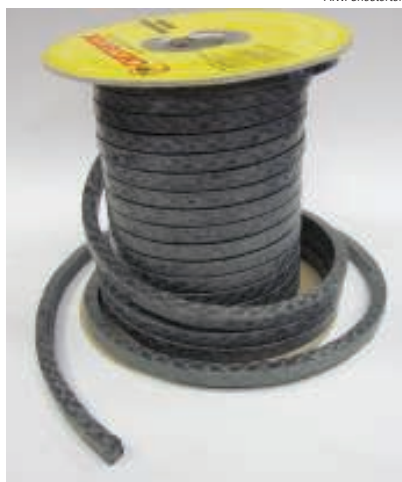
FIGURE 1. Certified Low-E valve packings, like Chesterton 1622 valve packing, can help reduce fugitive emissions from valves. This high-performance, graphite valve-stem packing blocks valve fugitive emissions to below consent-decree requirements
