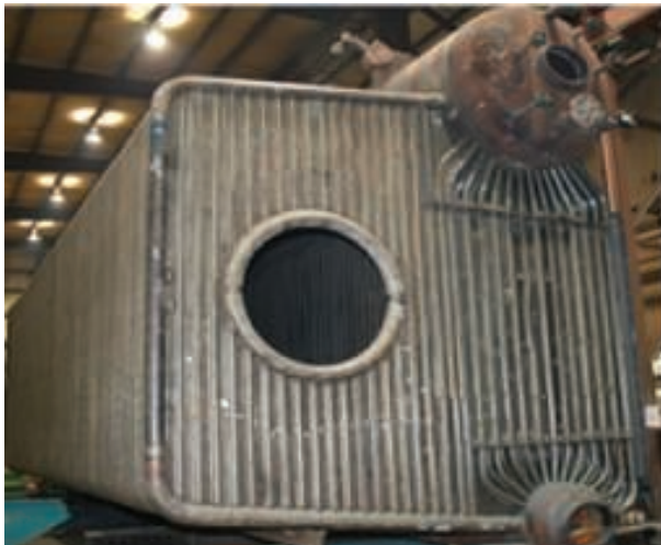
FIGURE 2. Completely water-cooled furnaces, such as the one shown here, help lower NOx emission and increase furnace effectiveness
