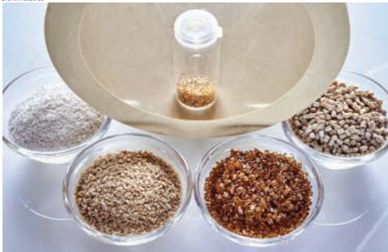
FIGURE 2. Evonik's Vestakeep 5000, a ductile polyetheretherketone (PEEK), is available as a granule for injection molding and extrusion to fulfill the design challenges for seals and gaskets. A recent development on that initial material, Vestakeep 5000 HCM, can also be adapted to improve the sliding and wear resistance needed in some applications
